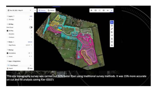
During earthworks Red Air Media can precisely measure the actual volume of spoil piles using 3D scanning software allowing contractors to more accurately plan for materials that need to be removed from site, leading to more correct up front cost planning.
